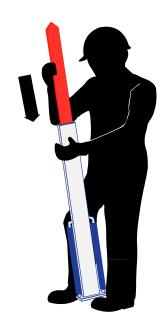
Remove marker from packaging and insert into post driver with the pointed end up.
