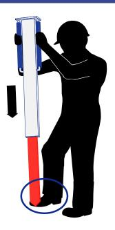
Drive marker into the ground with light taps, placing your foot against the base of the post to prevent the marker from flexing during installation.
