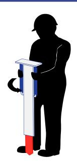
Rotate driver and marker 180°. Align marker so the decal or sheeting is facing the direction of traffic.
